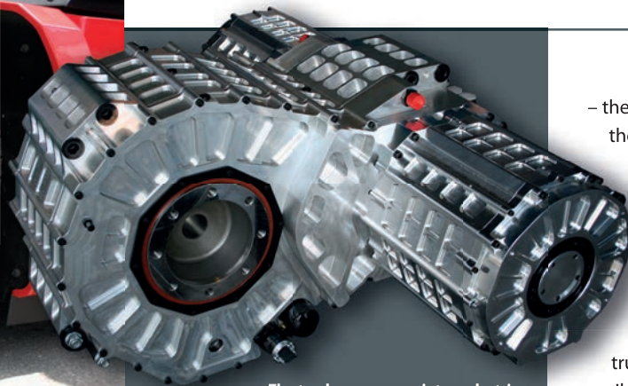
The trucks use a proprietary electric axle with a motor for each wheel.
